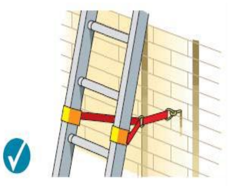
Tying near the base
