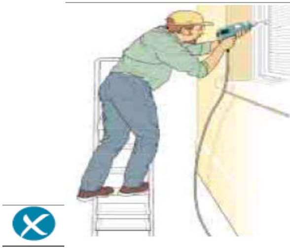
Incorrect – steps side on to work activity
